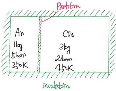
\* Determine the final temperature and pressure.
